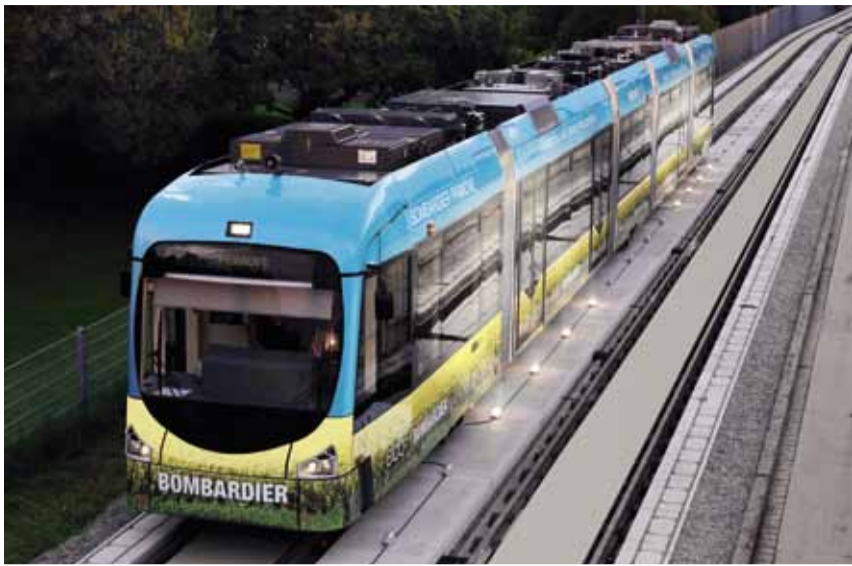
Tram equipped with BOMBARDIER PRIMOVE technology for contactless and catenary-free operation on the pilot line in Augsburg, Germany
